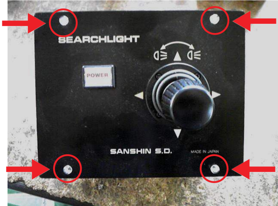
PICTURE 35 (Remote control panel CPF99)
